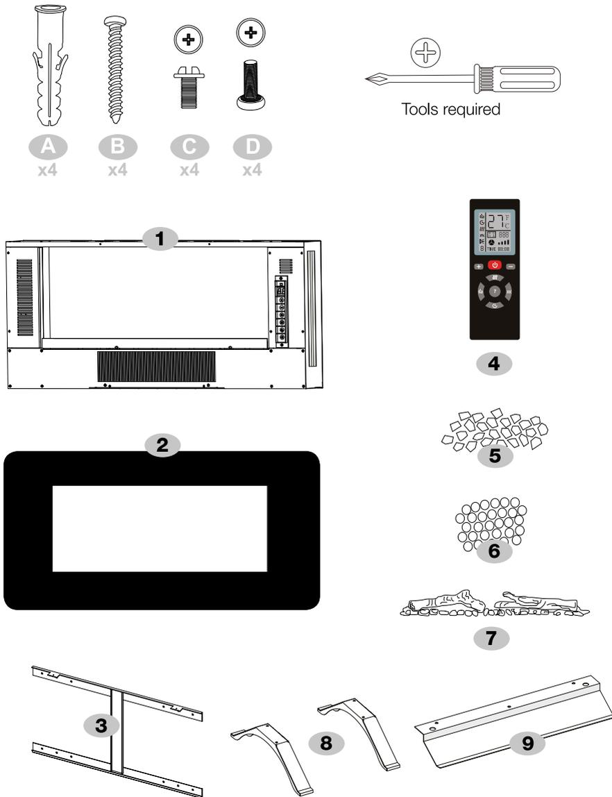
Ensure if wall-mount installation "baffle 9" is retained safely as it MUST be used for "On feet installation" if required in the future.
