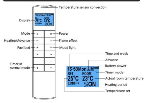
NOTE: This is a thermostatic remote control. The remote should be in the same room as the fireplace and placed on a flat surface. It must be placed away from the fire so the hot air will not blow on it and affect the thermostatic reading.
