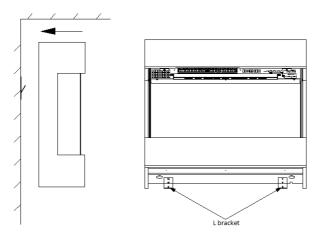
5.3e Drill two holes with 8mm drill bit on the marked place and install two plastic wall plugs. Fix the fireplace again on the bracket. Use two ST5\*40 screws to fix the L brackets on the wall.
