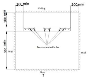
5.3c Tap the plastic wall plug into the six holes. Then use five ST5\*40 screws to fix the brackets on the wall.
