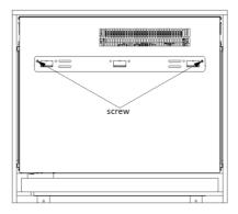
5.3b Choose a solid wall and mark six holes using the holes on the brackets. Drill the marked position using a suitable sized drill bit for the chosen fixings.
