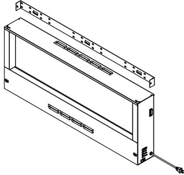
**2.2** Drill the four marked holes using an 8 mm drill. Tap the plastic dowels into the holes. If the wall is made from solid wood, it is not necessary to drill the holes or use the plastic dowels. Next, attach the wall bracket using 8 screw (ST5 x 40).
