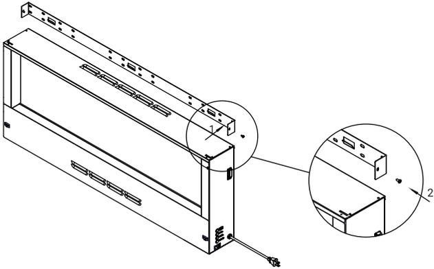
2.4 Hang the glass pane to the fire chamber, press the front of the glass and attach it to the surface of the fire chamber using 2 screws (M4 x 8).
