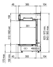
For the e-MatriX series, whilst stocks last, the fire casing may be 32mm lower than noted on the drawings in these brochures. After delivery, check the height of the fire casing to prevent misunderstandings. The very latest drawings of Faber fires are available on the website
