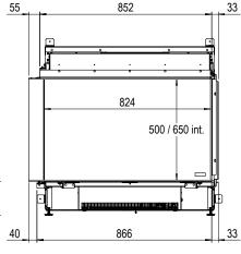
For the e-MatriX series, whilst stocks last, the fire casing may be 32mm lower than noted on the drawings in these brochures. After delivery, check the height of the fire casing to prevent misunderstandings. The very latest drawings of Faber fires are available on the website www.faberfires.com
