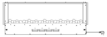
5.7 Hang the flat panel glass on the fire, and secure it with 2pcs ST4X10 screws.
