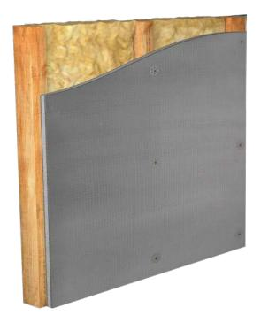
**WATERPROOFING:** To attain waterproof joints the boards should be sealed during installation using silicone sealant. The sealant should be applied to the edge of the fixed board immediately prior to the next board being installed and placed in position.
