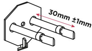
Fit the remaining energy cells to the bottom row, being careful not to damage or dislodge the element.
