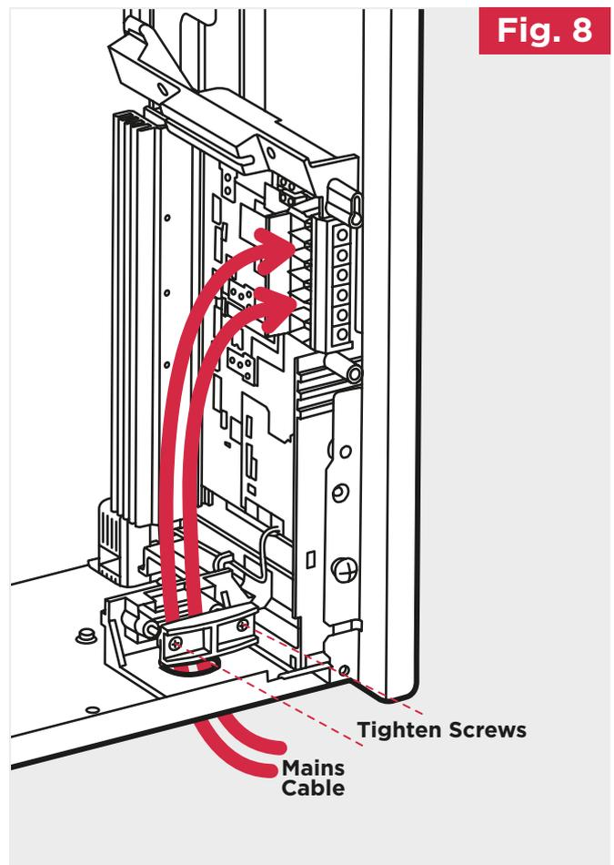
**8.** The mains cable entry and terminal block will be visible on the right hand side of the unit. Insert the mains cables through the cable gland at the bottom of the heater in readiness for connection (**Fig. 8**).
