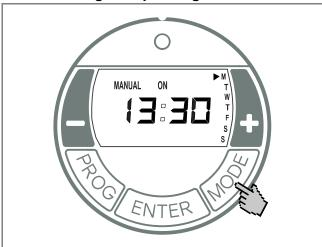
Pressing the MODE key switches the operating mode between MANUAL ON, MANUAL OFF and AUTO.
