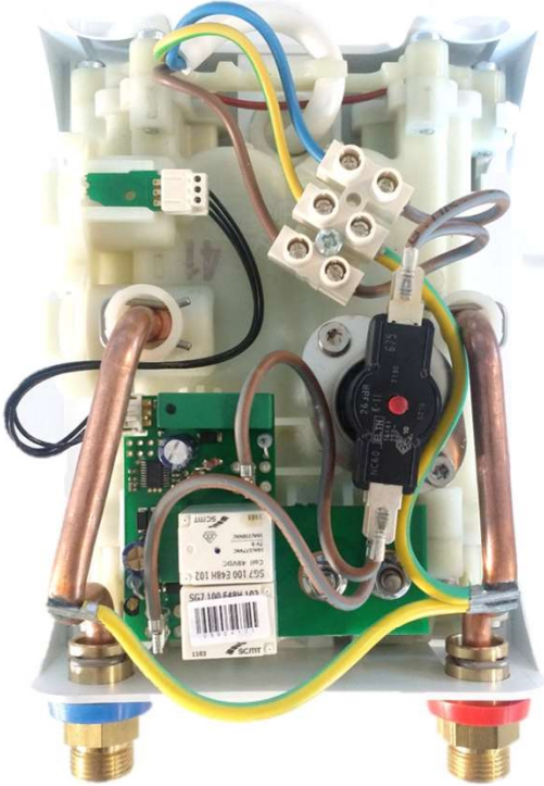
Bare-wire heating unit
